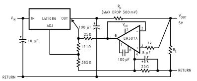
Figure 28. Remote Sensing
