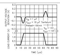
Figure 12. Load Transient Response
