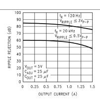
Figure 8. Ripple Rejection vs Output Current (LM1086-ADJ)
