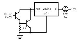
Figure 24. High Current Lamp Driver Protection
