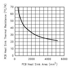
Figure 31. Heat Sink Thermal Resistance vs Area
