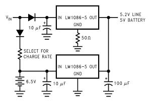
Figure 25. Battery Backup Regulated Supply
