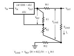
Figure 15. Best Load Regulation Using Adjustable Output Regulator
