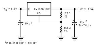
Figure 19. Adjustable at 5 V
