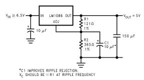
Figure 26. Ripple Rejection Enhancement
