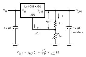
Figure 16. Basic Adjustable Regulator
