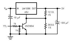
Figure 20. 5-V Regulator with Shutdown
