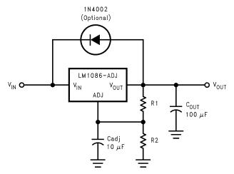
Figure 17. Regulator with Protection Diode
