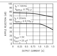
Figure 10. Ripple Rejection vs Output Current (LM1086-5)
