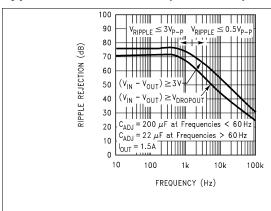
Figure 7. Ripple Rejection vs Frequency (LM1086-ADJ)
