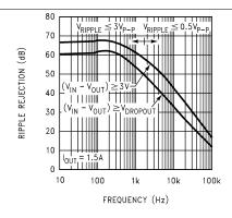
Figure 9. Ripple Rejection vs Frequency (LM1086-5)
